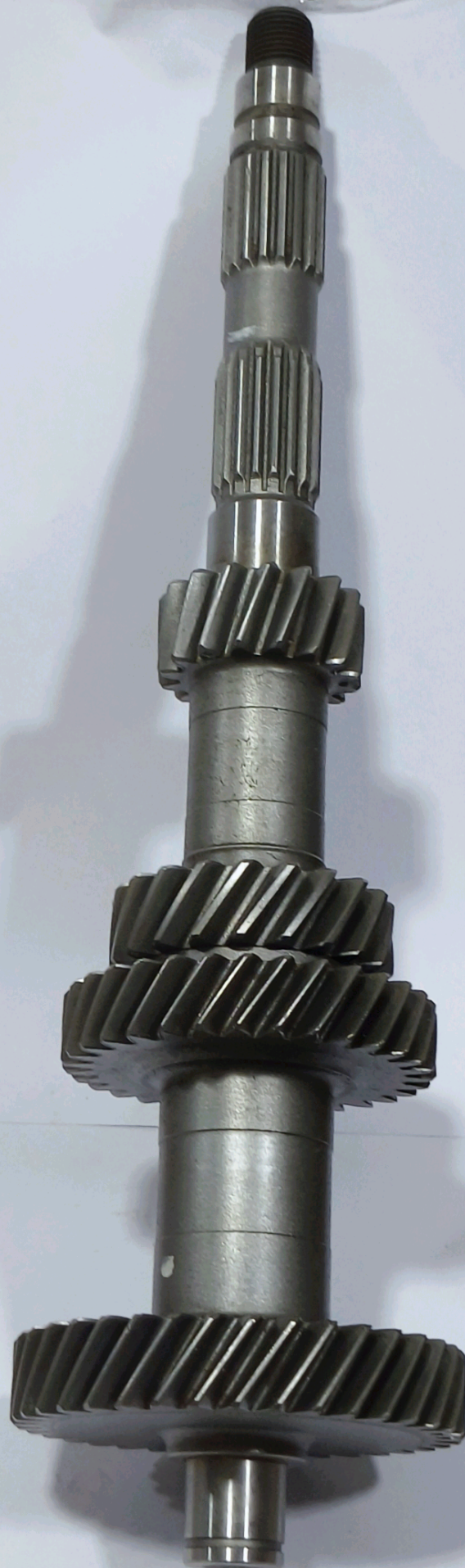
COUNTER GEAR DOST AVTEC 37,31,20,16 TEETH
