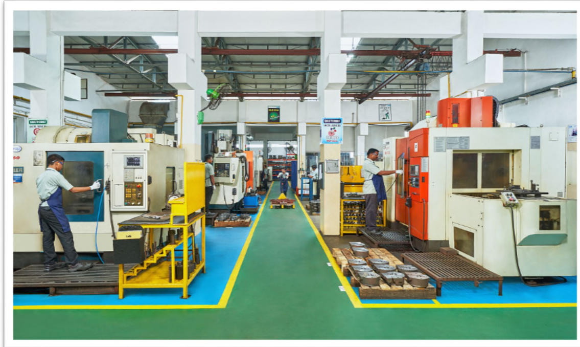
Precision machine shop with bank of VMC, CNC
